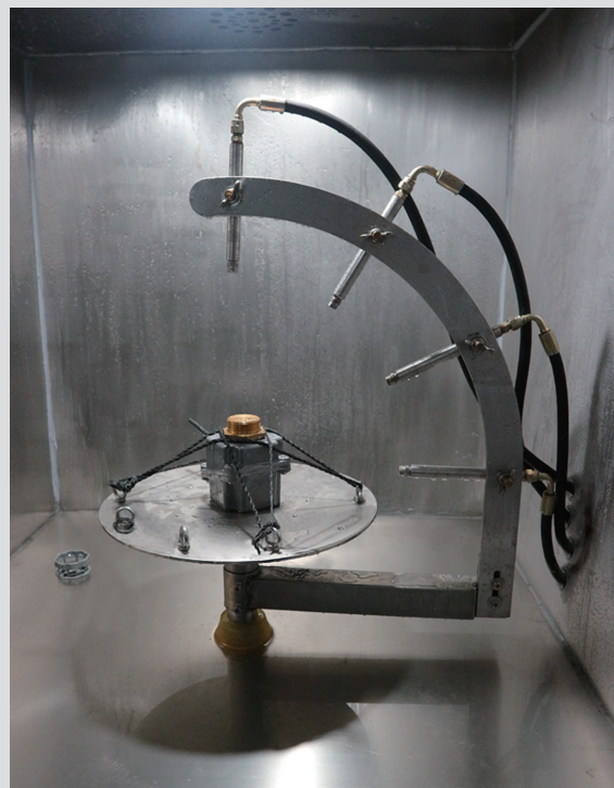
Enclosure during IPx9k test
