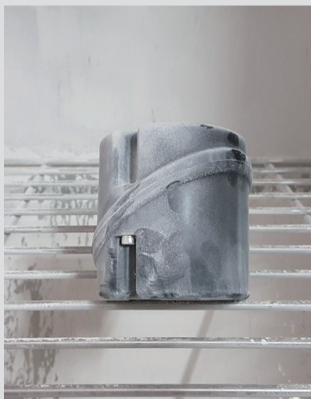
Enclosure during IP6x test
